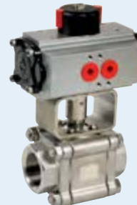
703 - Pneumatic actuated stainless steel ball valve (BSP) CF8M body & ball - TS: -30°C/+218°C.
