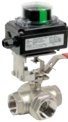
780 XS - Stainless steel - L port CF8M body - PTFE seats - Reduced bore - PS: 40 bar - TS: -10°C/+140°C.
