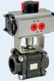
702 - Pneumatic actuated carbon steel ball valve (BSP) A216WCB body - CF8M ball - TS: -20°C/+218°C.
