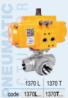
1370 L-port / 1370 T-port - Pneumatic actuated 3 way stainless steel ball valve (BSP) CF8M body - F316 ball - RTFE seats - Antistatic device - Reduced bore - PS: 69 bar - TS: -20°C/+180°C.
