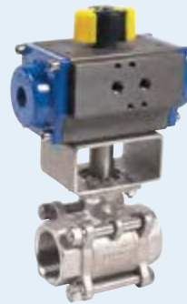
747 XS - Pneumatic actuated stainless steel ball valve (BSP) CF8M body & ball - TS: -40°C/+220°C
