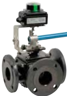
783 - Carbon steel - L port A216WCB body - PTFE seats - Full bore - PS: 16 bar - TS: -20°C/+150°C.
