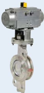
1116 - Pneumatic actuated stainless steel double offset butterfly valve CF8M body & disc - PS: 20 bar - TS: -10°C/+210°C - ⚠ Max. ΔP: 20 bar.
