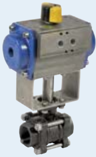
737 XS - Pneumatic actuated carbon steel ball valve (BSP) A216WCB body - CF8M ball - TS: -25°C/+220°C.
