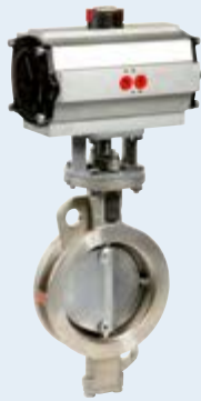
1116 - Pneumatic actuated stainless steel double offset butterfly valve CF8M body & disc - PS: 20 bar - TS: -10°C/+210°C - ⚠ Max. ΔP: 20 bar.
