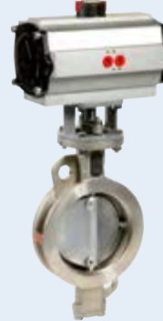
1116 - Pneumatic actuated stainless steel double offset butterfly valve CF8M body & disc - PS: 20 bar - TS: -10°C/+210°C - ⚠ Max. ΔP: 20 bar.
