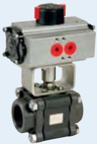
702 - Pneumatic actuated carbon steel ball valve (BSP) A216WCB body - CF8M ball - TS: -20°C/+218°C.
