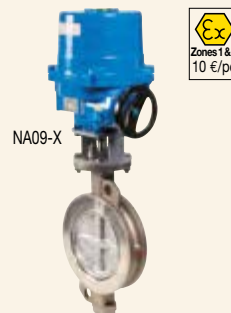
1116 - Electric actuated stainless steel double offset butterfly valve CF8M body & disc - PS: 20 bar - TS: -10°C/+210°C - ⚠ Max. ΔP: 20 bar.
