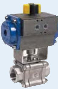
703 - Pneumatic actuated stainless steel ball valve (BSP) CF8M body & ball - TS: -30°C/+218°C.
