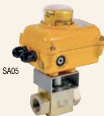
799 ZI - Electric actuated stainless steel ball valve F316 body & ball - Max. ΔP: 100 bar
