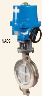
1116 - Electric actuated stainless steel double offset butterfly valve CF8M body & disc - PS: 20 bar - TS: -10°C/+210°C - ⚠ Max. ΔP: 20 bar.
