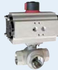
1370 L-port / 1370 T-port - Pneumatic actuated 3 way stainless steel ball valve (BSP) CF8M body - F316 ball - RTFE seats - Antistatic device - Reduced bore - PS: 69 bar - TS: -20°C/+180°C.
