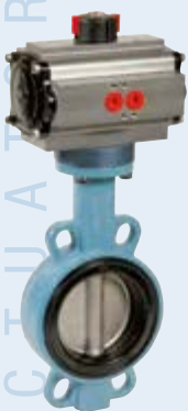
1147 - Pneumatic actuated ductile iron butterfly valve GGG50 disc (CF8M disc up to DN100) - Carboxylated NBR seat - PS: 16 bar - TS: -10°C/+90°C.
