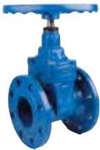
182 - NBR wedge - EN 558 series 14 (DIN 3202 F4) - With handwheel
