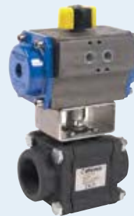
702 - Pneumatic actuated carbon steel ball valve (BSP) A216WCB body - CF8M ball - TS: -20°C/+218°C.
