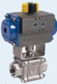
703 - Pneumatic actuated stainless steel ball valve (BSP) CF8M body & ball - TS: -30°C/+218°C.
