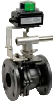
762 - Carbon steel A216WCB body - RTFE seats - Full bore - PS: 16 bar - TS: -20°C/+150°C.
