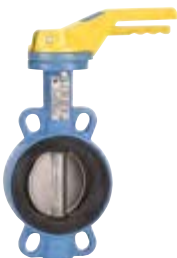
1141 - Disc CF8M up to DN100, Disc GGG50 epoxy coated above / Seat NBR For gas - PS: 5 bar (class MOP5) - TS: -20°C/+60°C.
