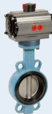
1147 - Pneumatic actuated ductile iron butterfly valve GGG50 disc (CF8M disc up to DN100) - Carboxylated NBR seat - PS: 16 bar - TS: -10°C/+90°C.
