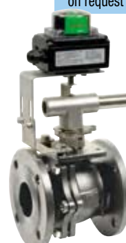
753 - Stainless steel CF8M body - RTFE seats - Full bore - PS: 16 bar - TS: -20°C/+200°C.
