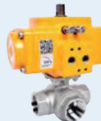
1370 L-port / 1370 T-port - Pneumatic actuated 3 way stainless steel ball valve (BSP) CF8M body - F316 ball - RTFE seats - Antistatic device - Reduced bore - PS: 69 bar - TS: -20°C/+180°C.
