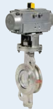
1116 - Pneumatic actuated stainless steel double offset butterfly valve CF8M body & disc - PS: 20 bar - TS: -10°C/+210°C - ⚠ Max. ΔP: 20 bar.
