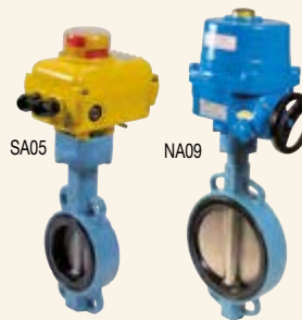
1158 - Electric ductile iron butterfly valve Aluminium bronze disc - NBR seat - PS: 16 bar - TS: -10°C/+80°C.
