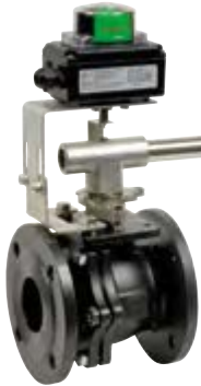
752 - Carbon steel A216WCB body - RTFE seats - Full bore - PS: 16 bar - TS: -20°C/+200°C.
