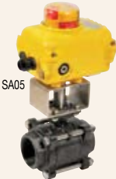
737 XS & 739 XS - Electric actuated carbon steel ball valve (BSP) (SW) A216WCB body - CF8M ball - TS: -25°C/+220°C.
