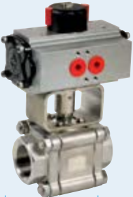
703 - Pneumatic actuated stainless steel ball valve (BSP) CF8M body & ball - TS: -30°C/+218°C.
